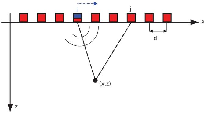
Fig. 1. Concept of TFM data acquisition. A single element is transmitting a pulse (in blue) and the signals are received by all transducers (in red). This operation is performed for all transmitting elements.
