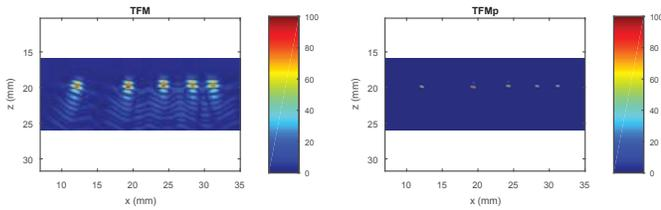
Fig. 4. Images obtained by TFM and TFMp for the second example. TFMp is tuned with  $\mu = 70\% \mu_{max}$ .
