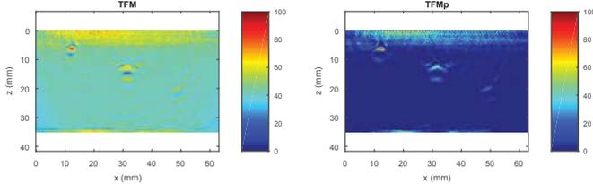
Fig. 5. Images obtained by TFM and TFMp for the third example. TFMp is tuned with  $\mu = 50\% \mu_{max}$ .
