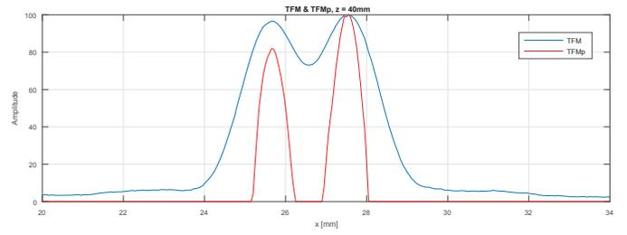
Fig. 3. Line for  $z = 40$  mm for the first example with two close reflectors.
