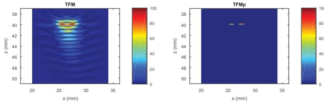
Fig. 2. Images obtained by TFM and TFMp for the first example with two close reflectors. TFMp is tuned with  $\mu = 80\% \mu_{max}$ .
